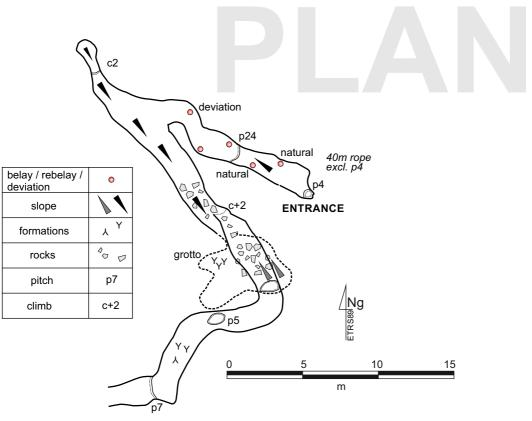
This cave survey is aligned to the ETRS89 grid which is 0.4 degrees to the west of True North.
