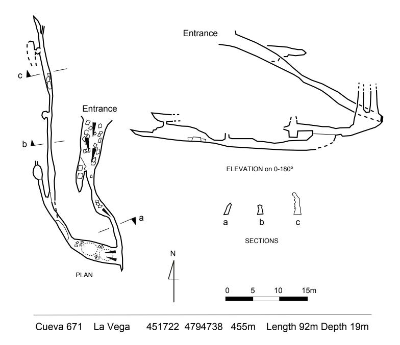
Surveyed August 2013 with compass and clinometer, estimating the lengths Drawn by PS
