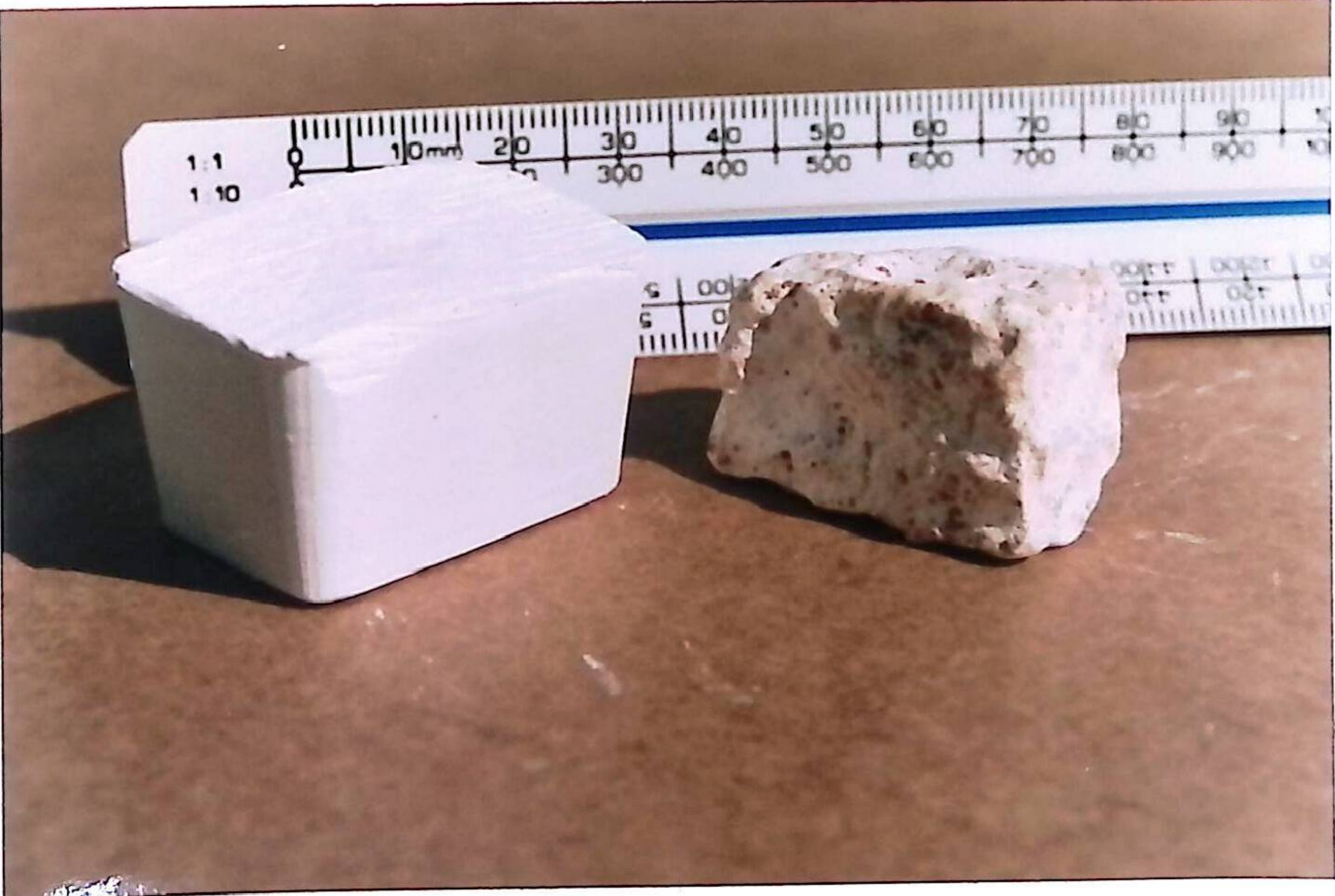
Figure 4:3 WEATHERED AND UNWEATHERED GYPSUM BLOCKS
